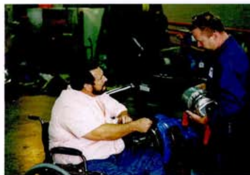
Bendix engineer Scott Wagner shows Barry Owens a new spring-loaded parking brake being installed in his truck
